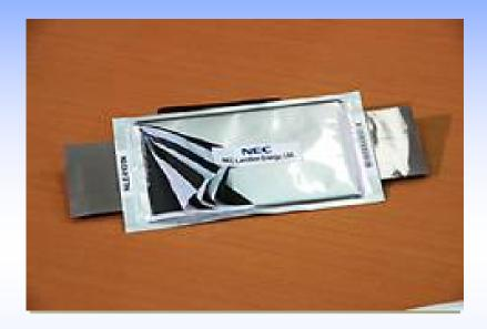
13.2 Ah, 25 cm long, 14 cm wide, and9 mm thick.Manganese-based positive.
